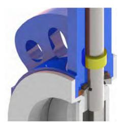
Disc spring, two sets for a group, is a state of compressive deformation in the body. It will impose elastic force on the press sleeve, compact the O ring and seat, improve axial sealing, then provided the bearing stress for the seat and disc, to cover the shortage of elasticity about PTFE seat.
